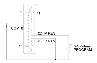
Figure 3-9. Remote Current Programming Using Resistance
