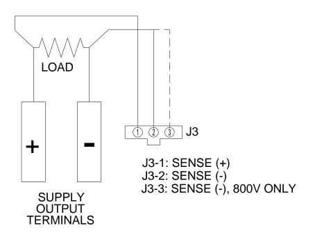
Figure 3-14. Remote Sensing Operation at the Load
