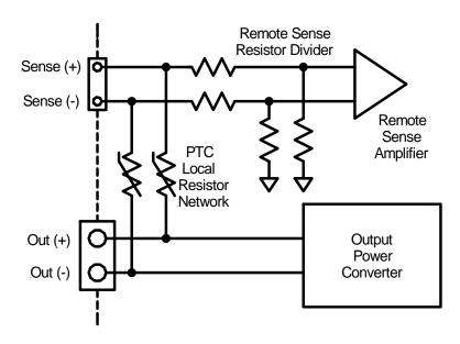
Figure 3-13. Local/Remote Voltage Sensing
