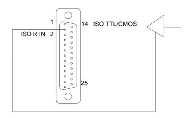
Figure 3-17. Remote Output ON/OFF Using Isolated TTL/CMOS Voltage Supply
