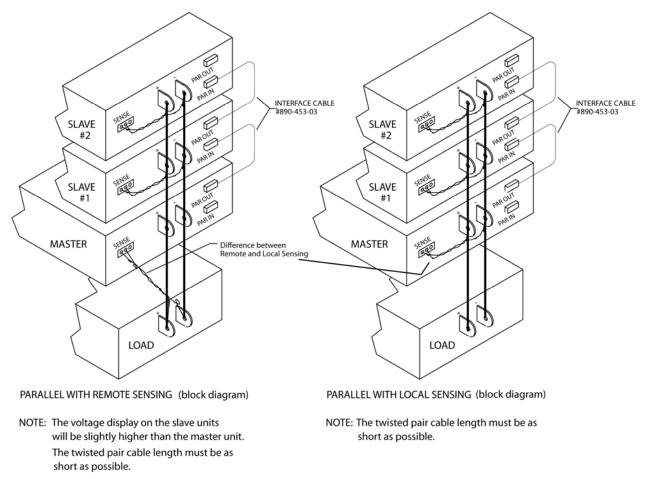
Figure 3-20. Parallel and Remote/Local Sense Connections
