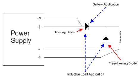
Figure 2-1. Diode Connection
