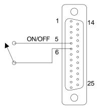
Figure 3-15. Remote Output ON/OFFControl by Contact Closure
