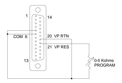
Figure 3-11. Remote Voltage Programming Using Resistance
