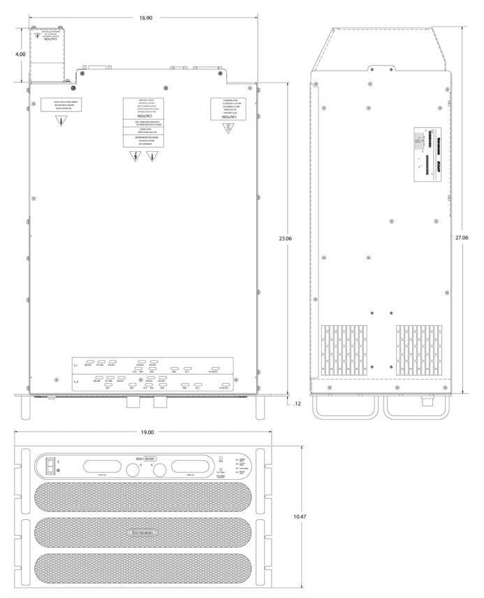
Figure 2-4. SGA Dimensions, 6U Models, 20kW to 30kW
