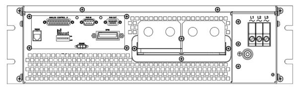
Figure 3-3. SG Rear Panel with GPIB Option (10V-300V)
