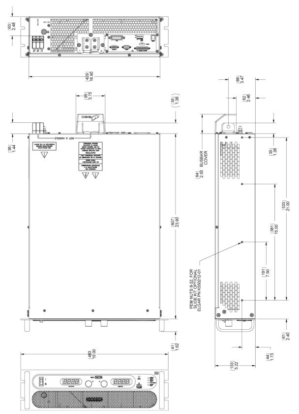
Figure 2-8. SGA Detailed Chassis Dimensions for Installation, Models 40V-600V
