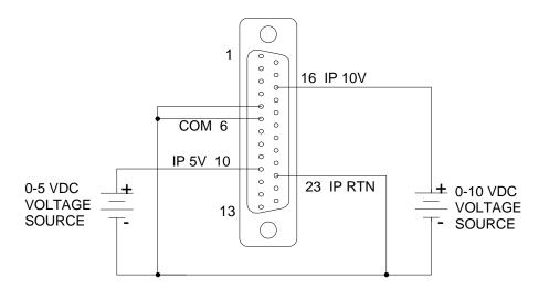
Figure 3-10. Remote Current Programming Using 0-5 or 0-10 VDC Voltage Source
