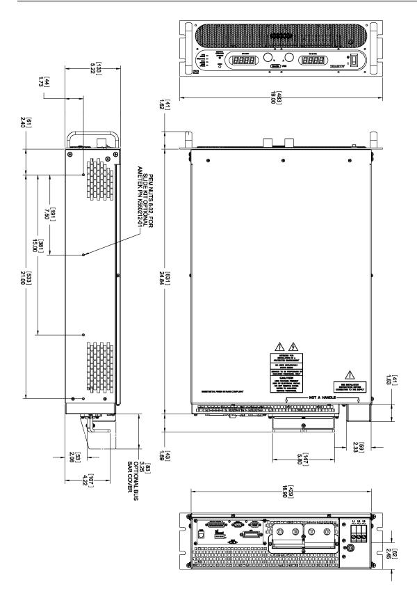
Figure 2-9. SGA Detailed Chassis Dimensions for Installation, Models 10V-30V
