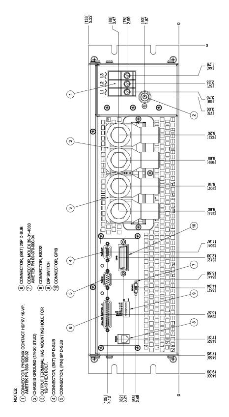
Figure 2-6. Rear Panel Input-Output Connector Locations, Models 10V-30V
